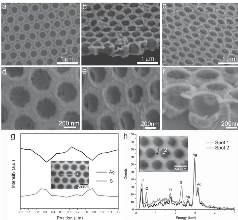
Figure 2. SEM images of  $\text{Ag}_2\text{S}$ -Ag heterostructured nanobowl arrays before (a,b) and after (c-f) removal of MCC template. EDS analysis results: (g) elemental profiles of line scanning, (h) EDS spectra of two selected spots.
