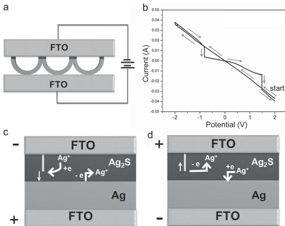
Figure 3. Schematic structure (a) and  $I$ - $V$  curve (b) of FTO/Ag/ $\text{Ag}_2\text{S}$ /FTO device made of the heterostructured nanobowl arrays. (c,d) Schematic illustration of the operating mechanism.
