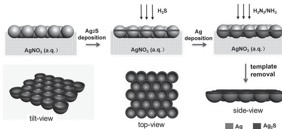
**Figure 1.** Schematic illustration of the fabrication of  $\text{Ag}_2\text{S}$ -Ag heterostructured nanobowl arrays by two-step nanosphere lithography at the gas-liquid interface.
