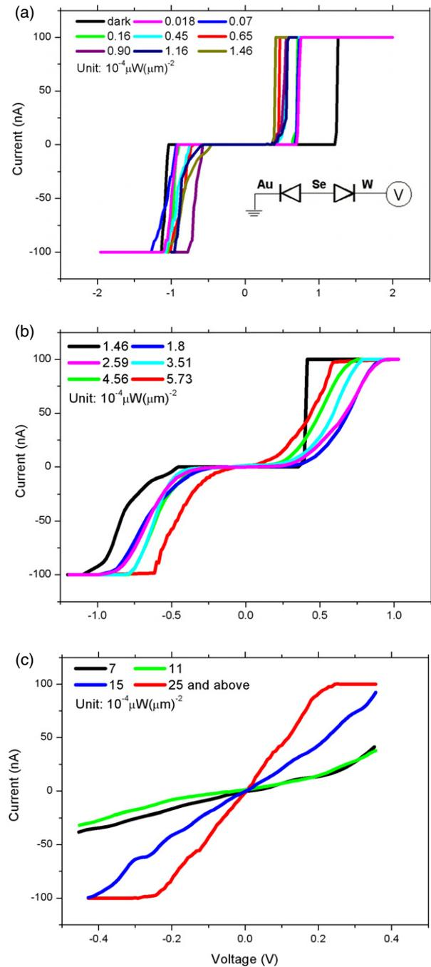
**Figure 3.**  $I(V)$  characteristics of SCSNT under different illumination intensities. The inset shows an equivalent device model of two back-to-back Schottky barrier diodes.
