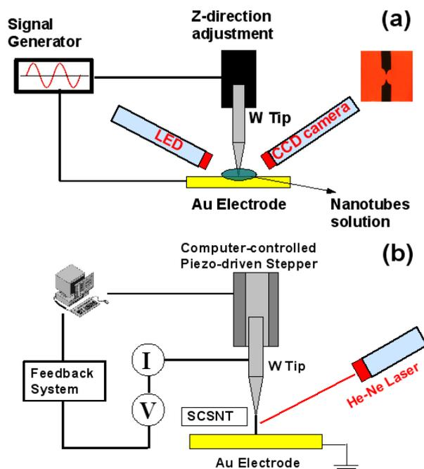
**Figure 2.** Schematics of (a) dielectrophoresis apparatus used to attach single SCSNT to a metal tip and (b) a single SCSNT two-terminal device arrangement for photoconductivity measurement.
