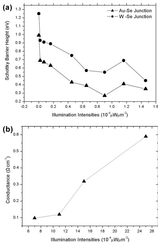
**Figure 5.** (a) Schottky barrier heights of Au–Se and W–Se contact under low-power illumination; (b) photoconductivity of Au–Se–W device under low-power illumination.
