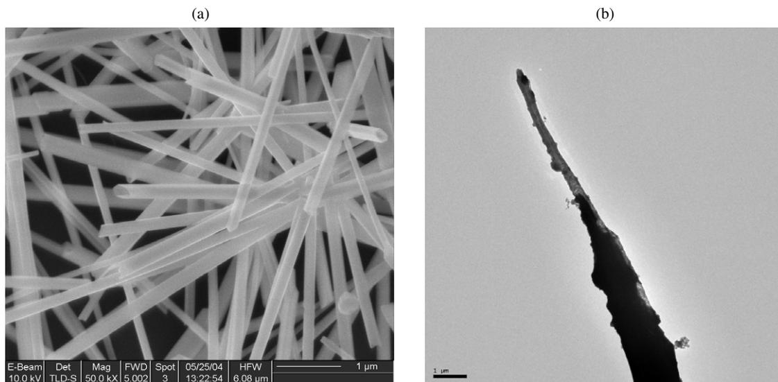
**Figure 1.** (a) SEM image of single-crystalline Se nanotubes as synthesized; (b) TEM image of an SCSNT attached to a tungsten tip.
