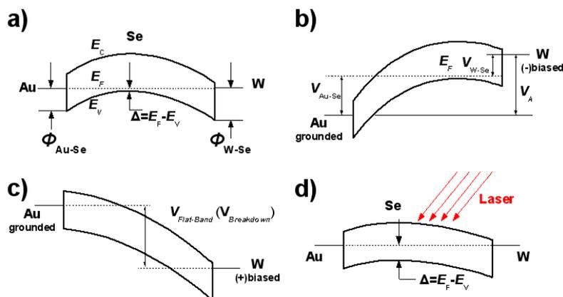
**Figure 4.** Energy band diagram of Au–Se–W device (a) in equilibrium state with zero bias and under dark conditions; (b) under the low-bias condition, showing band bending; (c) under the high-bias condition, showing reverse junction breakdown; and (d) under light illumination which reduces the barrier heights.
