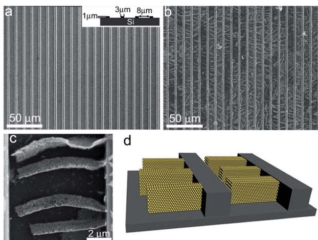
Fig. 6 (a) SEM image of the patterned substrate with parallel raised stripes. The inset schematically shows the side view of the substrate with the structural parameters labelled. (b and c) SEM images of the nearly parallel supercrystalline microplates assembled from GNRs. (d) Schematic illustration of parallel supercrystalline microplates standing on the trenches.
