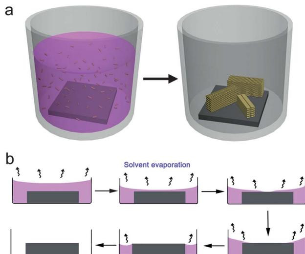
Fig. 1 (a) Schematic illustration of the experimental setup for self-assembly of GNRs via bulk solution evaporation. (b) Schematic side view of continuous decline of the solution surface with a concave meniscus upon solvent evaporation.
