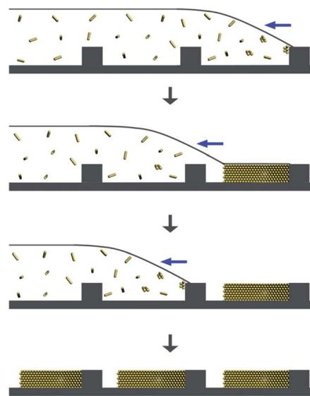
Fig. 7 Schematic illustration of the formation of vertically aligned, supercrystalline microplates perpendicular to the parallel stripes, showing the nucleation on the right walls of the trenches and the subsequent growth accompanying the gradual movement of the contact line. Blue arrows refer to the direction of contact line movement.
