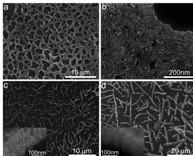
Fig. 3 SEM images of GNR assemblies obtained in aqueous GNR dispersions with different GNR concentrations: (a and b) net-like monolayer assemblies obtained at 1.6 nM ([CTAB] = 1 mM); (c) branch-like assemblies obtained at 4 nM ([CTAB] = 1 mM); (d) long-plate-like supercrystals obtained at 20 nM ([CTAB] = 2.5 mM). Insets in (c) and (d) are the enlarged SEM images showing the packing structure of GNRs.
