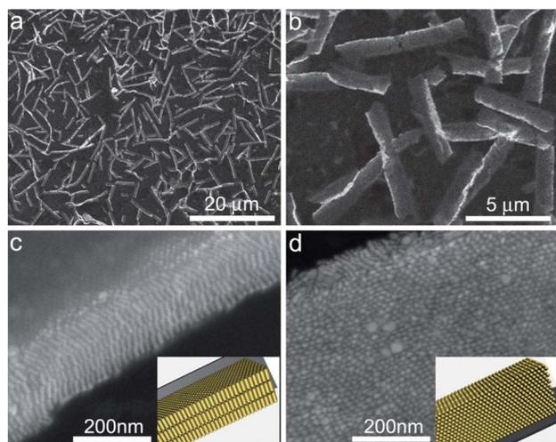
Fig. 2 (a and b) SEM images of vertically aligned, supercrystalline microplates assembled by GNRs ([GNR] = 8 nM, [CTAB] = 1 mM). (c) SEM image of an upstanding microplate showing the lying nanorods aligned in a smectic way. (d) SEM image of a tilted microplate showing the hexagonally packed, standing nanorods. Insets of (c) and (d) are the related 3D simulation models of the supercrystalline microplates viewed along different observation angles.
