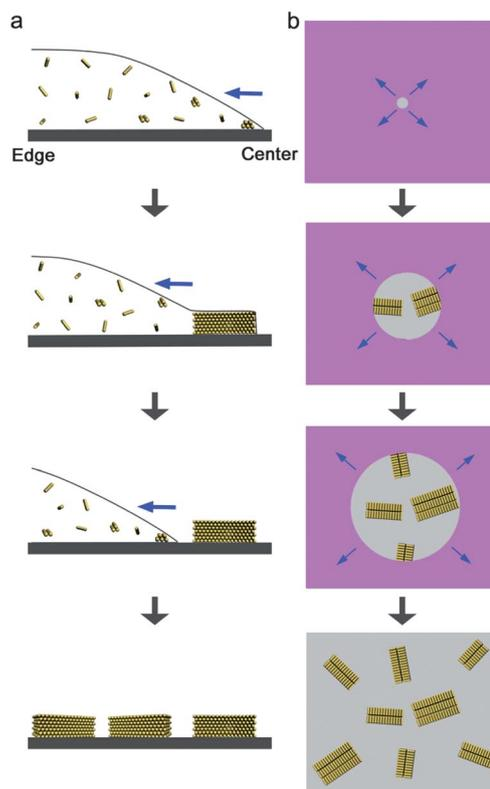
Fig. 4 Schematic illustration of the formation of vertically aligned, supercrystalline microplates via bulk solution evaporation with a continuously receding contact line. Side view (a) and top view (b) of the gradual movement of the contact line and the concomitant formation of plate-like supercrystals. Blue arrows refer to the direction of contact line movement.
