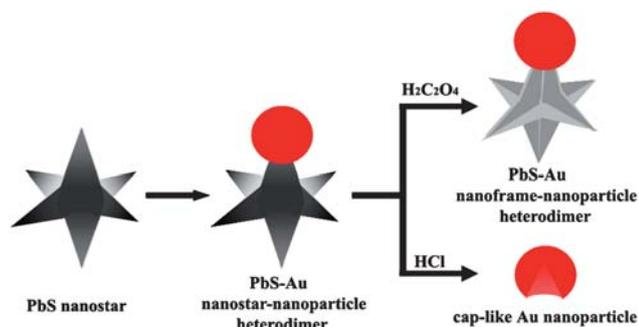
**Scheme 1** Schematic illustration of the formation of a PbS–Au nanostar–nanoparticle heterodimer and its transformation into a PbS–Au nanoframe–nanoparticle heterodimer and cap-like Au nanoparticle by acid etching.
