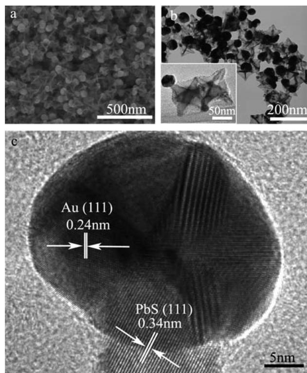
**Fig. 6** SEM (a), TEM (b), and HRTEM (c) images of PbS–Au nanoframe–nanoparticle heterodimers obtained by etching the PbS–Au nanostar–nanoparticle heterodimers formed with  $[\text{PbS}] = 0.48$  mM using 0.05 M oxalic acid.
