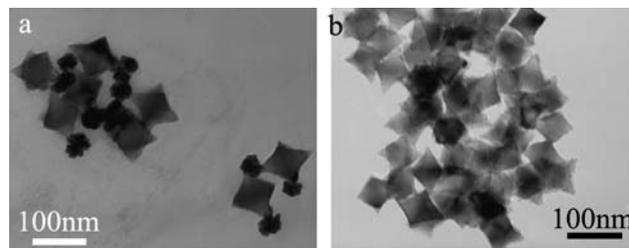
**Fig. 4** TEM images of PbS-Au nanostar-nanoparticle heterostructures formed with  $[\text{PbS}] = 0.48$  mM at 4 °C (a) and 60 °C (b).
