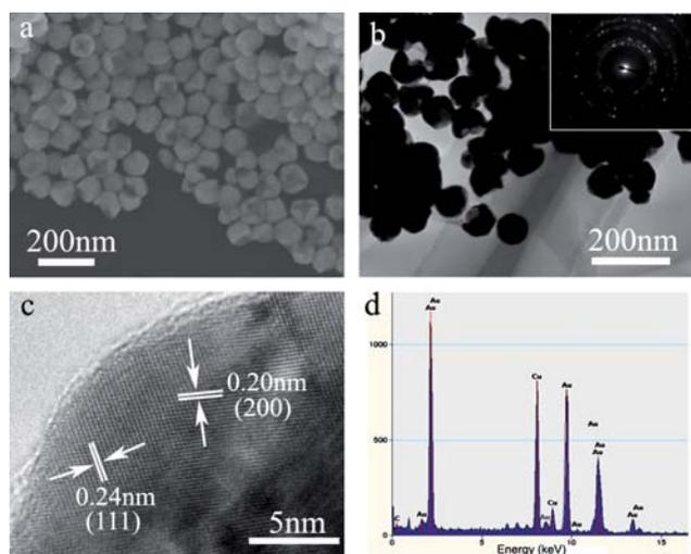
**Fig. 7** SEM (a), TEM (b), and HRTEM (c) images and EDS spectrum (d) of cap-like Au nanoparticles obtained by etching the PbS–Au nanostar–nanoparticle heterodimers formed with  $[PbS] = 0.08$  mM using 6 M HCl. The inset shows the related ED pattern.
