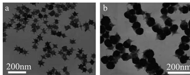
**Fig. 5** TEM images of PbS nanostars with sharp horns (a) and their related PbS-Au nanostar-nanoparticle heterodimers (b).
