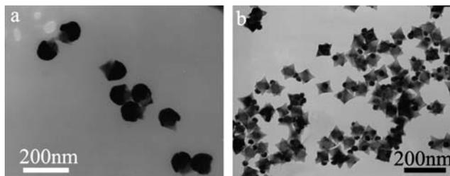
**Fig. 3** TEM images of PbS-Au nanostar-nanoparticle heterodimers formed at 27 °C with different PbS concentrations: (a) 0.08 mM and (b) 1.6 mM.
