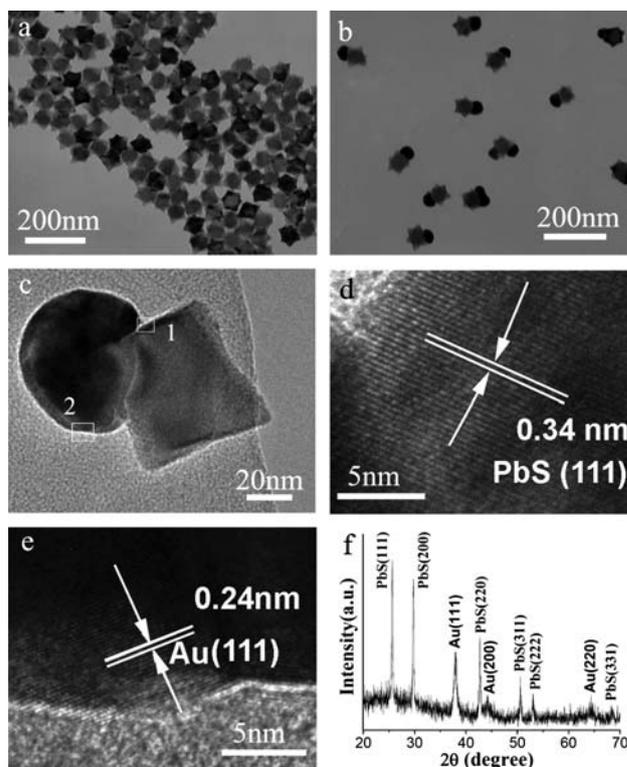
**Fig. 1** (a) A TEM image of PbS nanostars. (b), (c) TEM images, (d), (e) HRTEM images and (f) XRD pattern of PbS–Au nanostar–nanoparticle heterodimers formed with [PbS] = 0.48 mM at 27 °C. The HRTEM images shown in (d) and (e) correspond to the framed areas 1 and 2 in (c), respectively.
