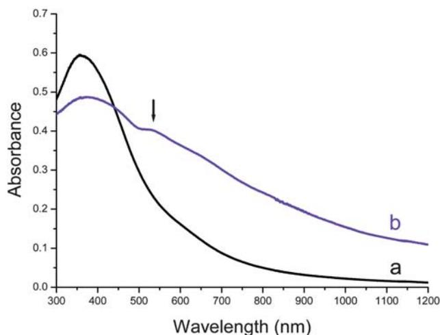
**Fig. 2** UV-vis spectra of PbS nanostars (a) and PbS-Au nanostar-nanoparticle heterodimers (b). The arrow indicates the SPR peak of Au nanoparticles grown on the PbS nanostars.
