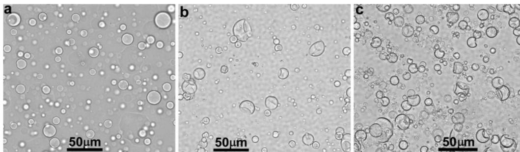
**Figure 5.** Optical micrographs of gigantic hollow shells of mesoporous silica obtained after different times of reaction: (a) 0 min; (b) 30 min; (c) 3 h. [CTAB] = 4.8 mM,  $r = 1.44$ ,  $x = 0.07$ .
