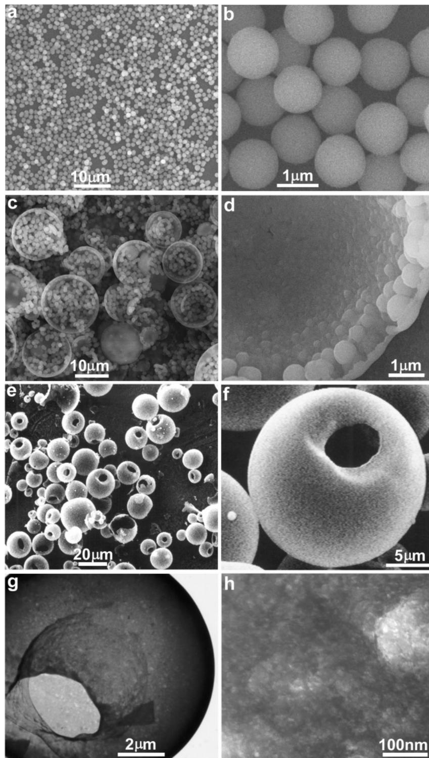
**Figure 1.** SEM (a–f) and TEM (g,h) images of mesoporous silica synthesized at different water-to-ethanol volume ratios ( $r$ ): (a,b) monodisperse microspheres obtained at  $r = 0.63$ ; (c,d) a mixture of microspheres and gigantic hollow shells composed of small spheres obtained at  $r = 0.95$ ; (e–h) gigantic hollow shells obtained at  $r = 1.44$ . [CTAB] = 4.8 mM, TEOS volume content  $x = 0.07$ .
