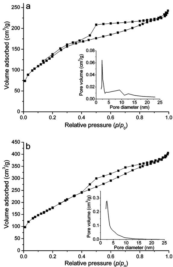
**Figure 2.** Nitrogen adsorption–desorption isotherms of mesoporous silica: (a) monodisperse microspheres obtained at  $r = 0.63$ ; (b) gigantic hollow shells obtained at  $r = 1.44$ . Insets show the pore size distribution determined from the adsorption branch. [CTAB] = 4.8 mM,  $x = 0.07$ .
