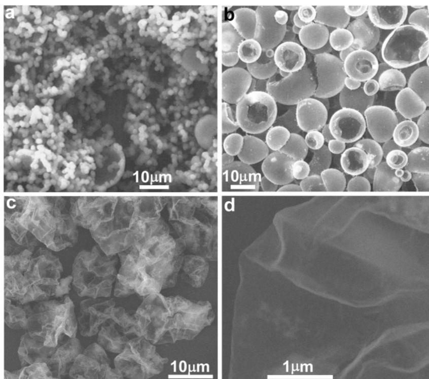
**Figure 4.** SEM images of mesoporous silica synthesized at different CTAB concentrations: (a) microspheres together with a few gigantic hollow shells obtained at [CTAB] = 13.3 mM; (b) gigantic hollow shells obtained at [CTAB] = 1.9 mM; (c,d) gigantic hollow capsules obtained at [CTAB] = 0.95 mM.  $r = 0.95$ ,  $x = 0.07$ .
