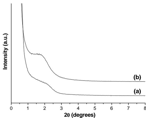
**Figure S1.** XRD patterns of mesoporous silica: (a) monodisperse microspheres obtained at  $r = 0.63$ ; (b) gigantic hollow shells obtained at  $r = 1.44$ . [CTAB] = 4.8 mM,  $x = 0.07$ .
