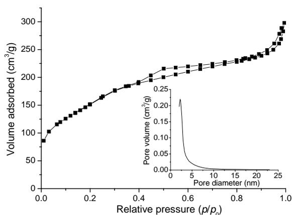
**Figure S2.** Nitrogen adsorption-desorption isotherms of bowl-like half shells of mesoporous silica obtained at  $x = 0.14$ . Inset shows the pore size distribution determined from the adsorption branch. [CTAB] = 4.8 mM,  $r = 0.95$ .
