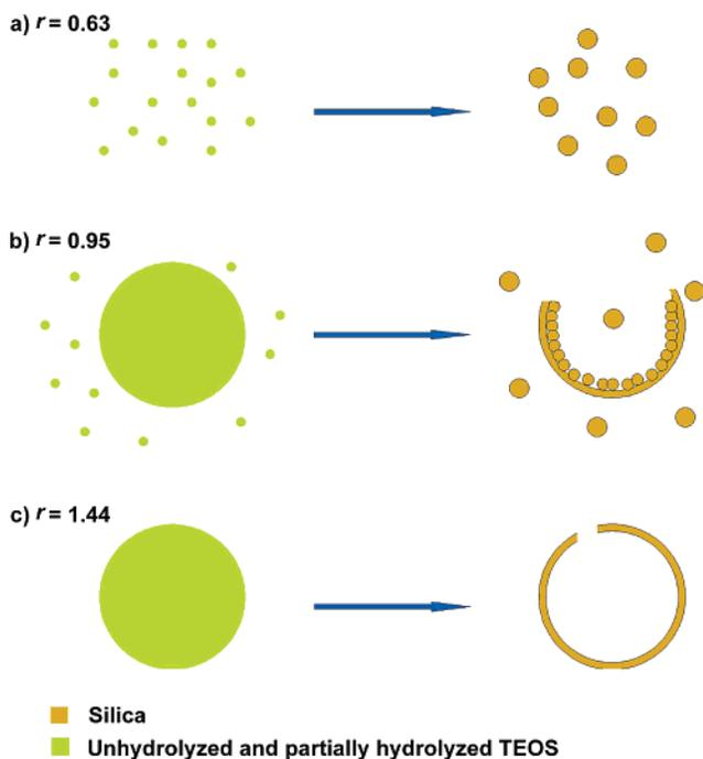
**Figure 6.** Schematic illustration of the morphology-controlled formation of mesoporous silica by adjusting the  $r$  values.
