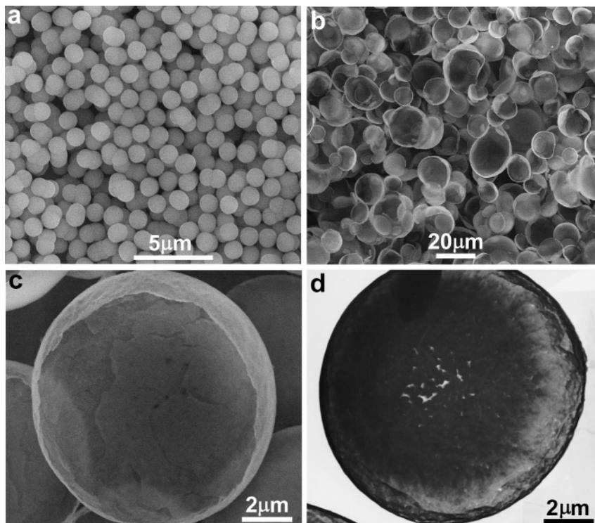
**Figure 3.** SEM (a–c) and TEM (d) images of mesoporous silica synthesized at different TEOS volume contents ( $x$ ): (a) monodisperse microspheres obtained at  $x = 0.04$ ; (b–d) bowl-like half shells obtained at  $x = 0.14$ . [CTAB] = 4.8 mM,  $r = 0.95$ .
