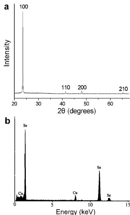
**Figure 2.** XRD pattern (a) and EDS spectrum (b) of Se nanobelts obtained in  $C_{18}EO_{20}$  micellar solution.
