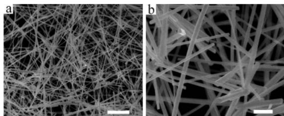
**Figure 3.** SEM images of Se nanowires obtained in  $C_{12}EO_{10}$  micellar solution. Scale bars: (a) 5  $\mu\text{m}$  and (b) 1  $\mu\text{m}$ .
