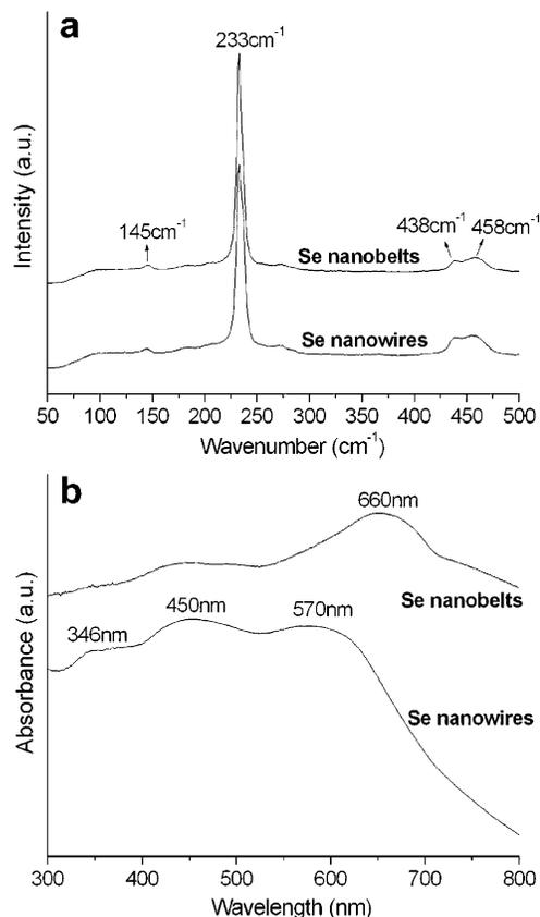
**Figure 4.** Raman scattering (a) and UV–vis absorption (b) spectra of Se nanobelts obtained in  $C_{18}EO_{20}$  micellar solution and Se nanowires obtained in  $C_{12}EO_{10}$  micellar solution.
