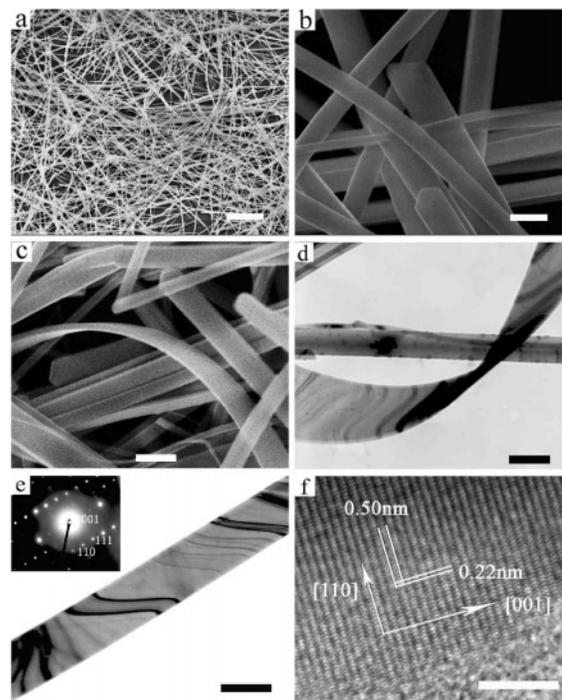
**Figure 1.** SEM (a–c), TEM (d–e), and HRTEM (f) images of Se nanobelts obtained in  $C_{18}EO_{20}$  micellar solution. The inset shows the related ED pattern. Scale bars: (a)  $5\ \mu m$ , (b–e) 200 nm, and (f) 5 nm.
