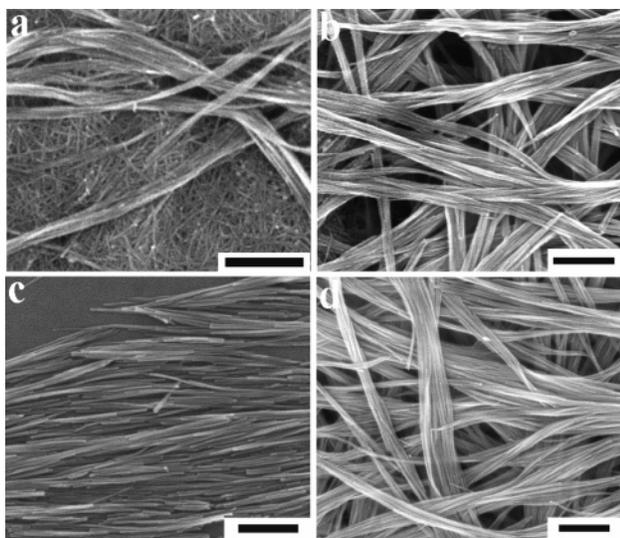
**Figure 3.** SEM images of  $\text{Cu}(\text{OH})_2$  nanowires prepared via the  $\text{KOH}/\text{NH}_3$  route aged for 2 min (a) and 1 h (b), and the  $\text{Cu}(\text{OH})_2$  nanowires obtained via the  $\text{KOH}/\text{NH}_3$  route aged for 1 h (c) and 12 h (d) and sonicated for 10 min. Scale bars: 500 nm.
