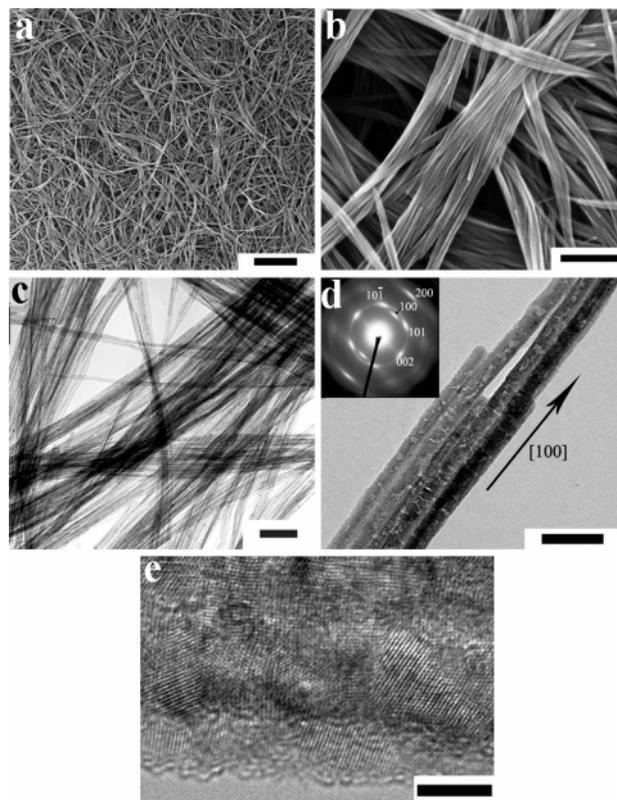
**Figure 1.** SEM (a, b), TEM (c, d), and HRTEM (e) images of  $\text{Cu}(\text{OH})_2$  nanowires prepared via the  $\text{KOH}/\text{NH}_3$  route aged for 12 h. Inset shows ED pattern of the bundled nanowires. Scale bars: (a)  $5\ \mu\text{m}$ ; (b)  $500\ \text{nm}$ ; (c)  $100\ \text{nm}$ ; (d)  $50\ \text{nm}$ ; (e)  $5\ \text{nm}$ .
