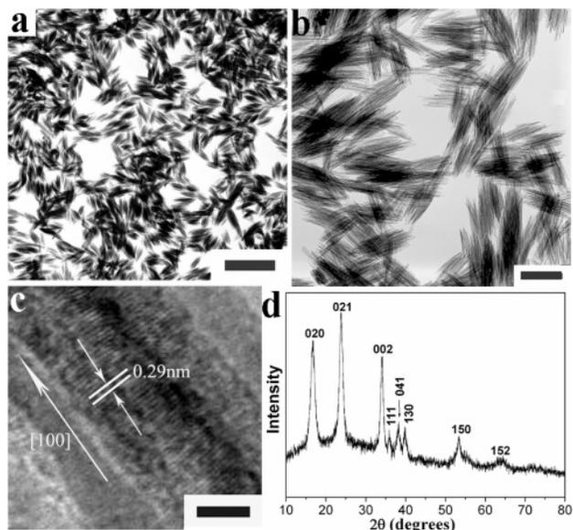
**Figure 5.** TEM (a, b) and HRTEM (c) images and the XRD pattern (d) of  $\text{Cu}(\text{OH})_2$  nanorod assemblies prepared via the  $\text{NH}_3/\text{KOH}$  route in the presence of PAA. Scale bars: (a) 1  $\mu\text{m}$ ; (b) 200 nm; (c) 3 nm.
