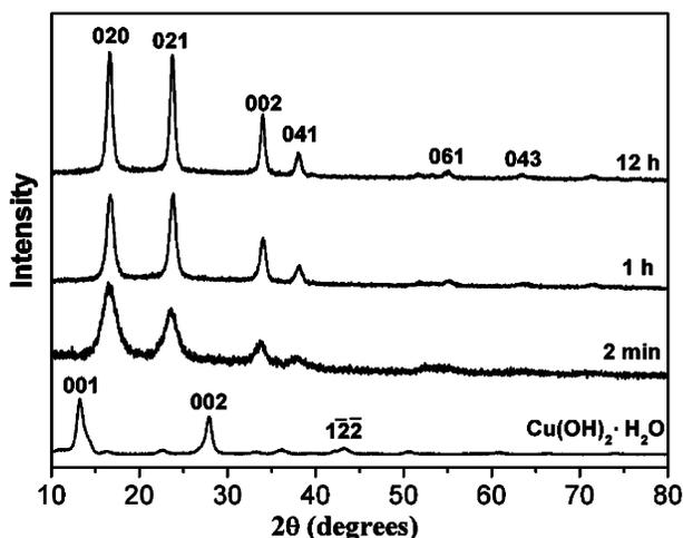
**Figure 2.** XRD patterns of  $\text{Cu}(\text{OH})_2$  nanowires prepared via the  $\text{KOH}/\text{NH}_3$  route aged for different periods. XRD pattern of  $\text{Cu}(\text{OH})_2 \cdot \text{H}_2\text{O}$  precipitates obtained before adding ammonia is also displayed.
