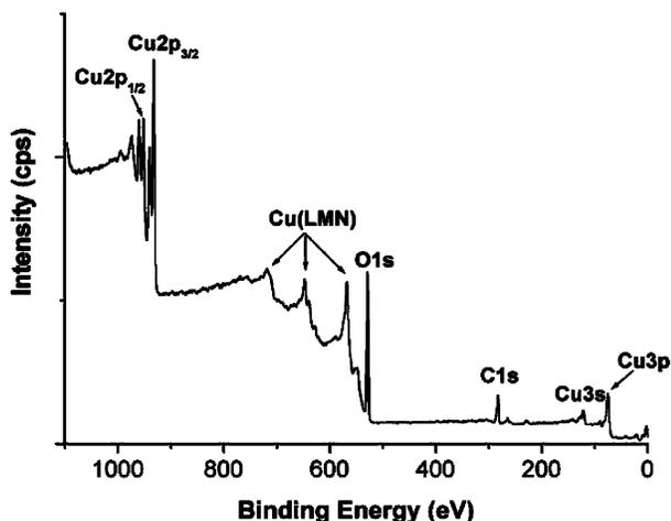
**Figure 6.** X-ray photoelectron spectrum of  $\text{Cu}(\text{OH})_2$  nanorod assemblies prepared via the  $\text{NH}_3/\text{KOH}$  route in the presence of PAA.
