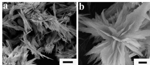
**Figure 9.** SEM images of CuO nanostructures obtained by thermal dehydration of the as-prepared Cu(OH)<sub>2</sub> nanoribbons in water at 70 °C for 12 h. Scale bars: (a) 2 μm; (b) 500 nm.
