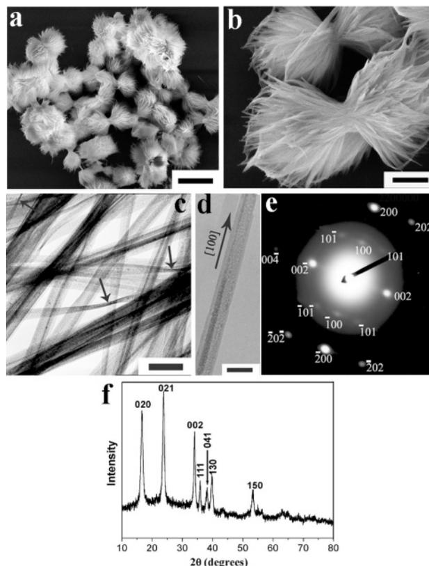
**Figure 4.** SEM (a, b) and TEM (c, d) images and ED (e) and XRD (f) patterns of  $\text{Cu}(\text{OH})_2$  nanoribbons prepared via the  $\text{NH}_3/\text{KOH}$  route. The ED pattern shown in plate e corresponds to the single nanoribbon shown in plate d. Scale bars: (a) 5  $\mu\text{m}$ ; (b) 1  $\mu\text{m}$ ; (c) 200 nm; (d) 100 nm.
