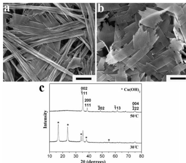
**Figure 7.** SEM images (a, b) and XRD patterns (c) of CuO nanoplatelets obtained by thermal dehydration of the  $\text{Cu}(\text{OH})_2$  nanowires prepared via the  $\text{KOH}/\text{NH}_3$  route immediately after the addition of the  $\text{KOH}$  and ammonia solutions: (a) 30 °C; (b) 50 °C. Scale bars: 500 nm.
