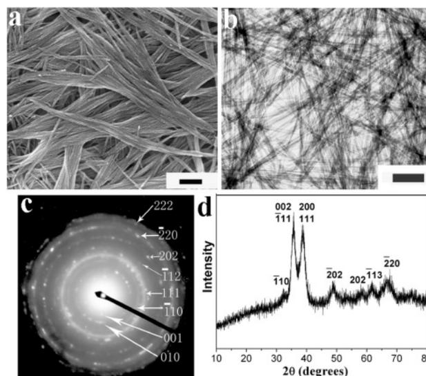
**Figure 10.** SEM (a) and TEM (b) images and ED (c) and XRD (d) patterns of CuO nanowires obtained by thermal dehydration of the as-prepared Cu(OH)<sub>2</sub> nanowires in the solid state at 120 °C for 2 h. Scale bars: (a) 500 nm; (b) 200 nm.
