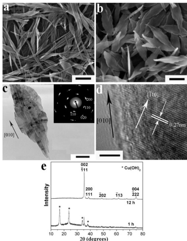
**Figure 8.** SEM (a, b), TEM (c), and HRTEM (d) images and XRD patterns (e) of CuO nanoleaflets obtained by thermal dehydration of the as-prepared Cu(OH)<sub>2</sub> nanowires in water at 70 °C for different times: (a) 1 h; (b–d) 12 h. Inset shows ED pattern of the single CuO nanoleaflet. Scale bars: (a, b) 500 nm; (c) 100 nm; (d) 3 nm.
