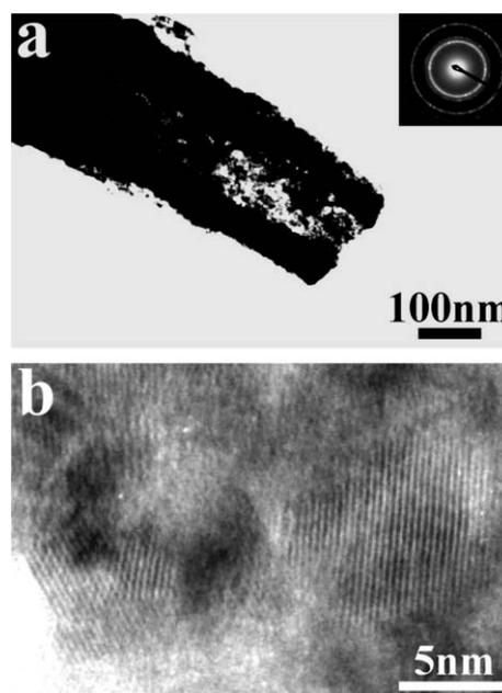
**Fig. 5** TEM (a) and HRTEM (b) images of  $\text{ZrO}_2$  tubes constituting the  $\text{ZrO}_2$  networks obtained at 600 °C.
