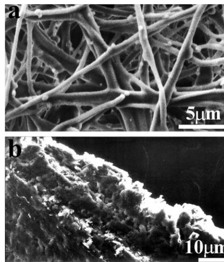
**Fig. 1** SEM images of the eggshell membrane (ESM) template. (a) Overview of the surface of ESM, (b) overview of the cross section of ESM.
