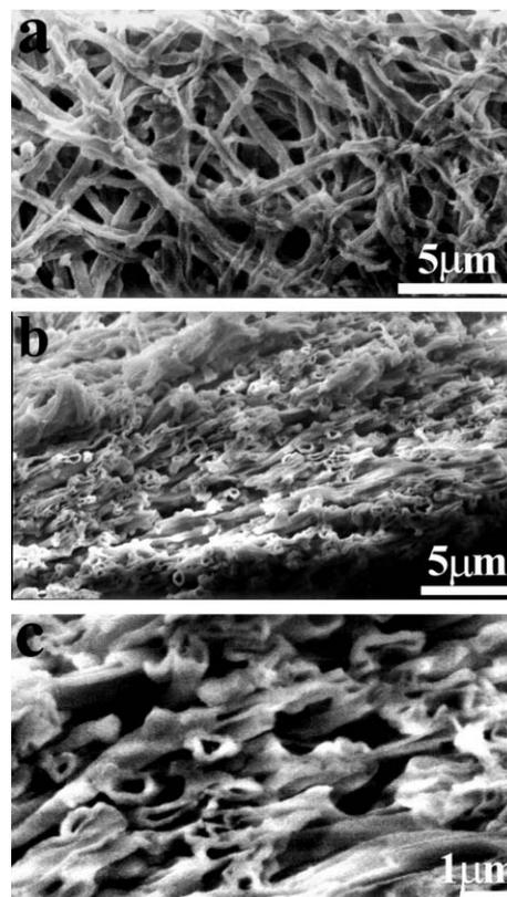
**Fig. 4** SEM images of ESM-templated  $\text{ZrO}_2$  networks obtained at 600 °C: a) overview of the surface, b) overview of the cross section, and c) higher magnification of the cross section showing the broken hollow tubes.
