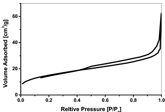
Fig. 6 Nitrogen adsorption-desorption isotherms of ESM-templated  $\text{ZrO}_2$  networks obtained at 600 °C.
