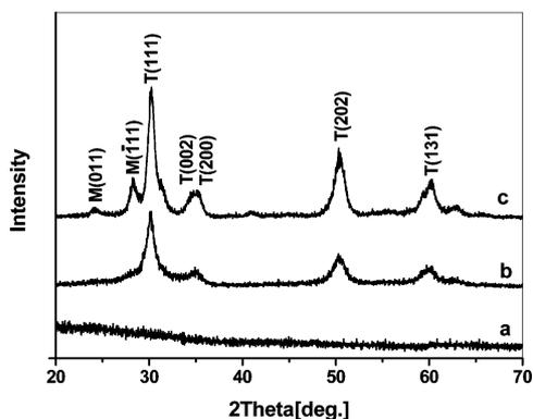
**Fig. 3** XRD patterns of ESM-templated  $\text{ZrO}_2$  samples: (a) as-synthesized ESM/ZP hybrid, (b)  $\text{ZrO}_2$  networks obtained at 600 °C, (c)  $\text{ZrO}_2$  networks obtained at 700 °C. T: tetragonal, M: monoclinic.
