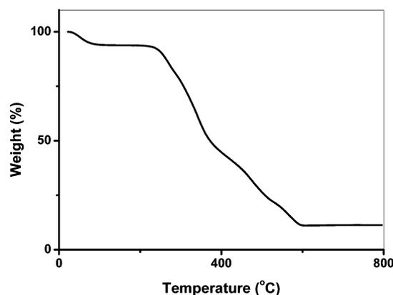
**Fig. 2** TGA curve of as-synthesized ESM/ZP hybrid.
