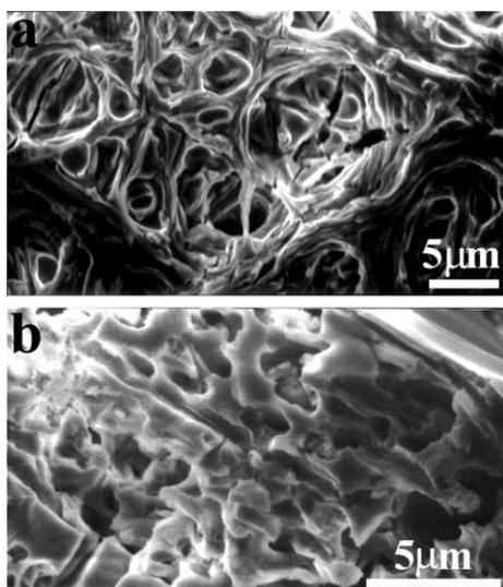
Fig. 7 SEM images of ESM-templated  $\text{ZrO}_2$  networks obtained at 700 °C: a) the surface, and b) the cross section.
