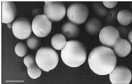
Fig. 7. SEM image of functionalized mesoporous silica spheres  $\text{SiO}_2\text{-2-C}_{18}$ . Scale bar: 5  $\mu\text{m}$ .
