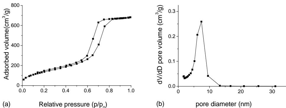
Fig. 9.  $N_2$  adsorption–desorption isotherm (a) and pore size distribution curve from the adsorption branch (b) of functionalized mesoporous silica spheres  $SiO_2$ -2- $C_{18}$ .
