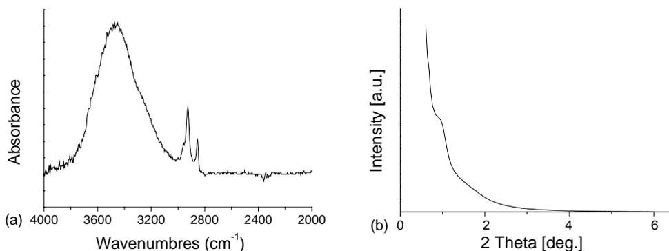
Fig. 8. IR (a) and XRD (b) spectra of functionalized mesoporous silica spheres  $\text{SiO}_2\text{-2-C}_{18}$ .
