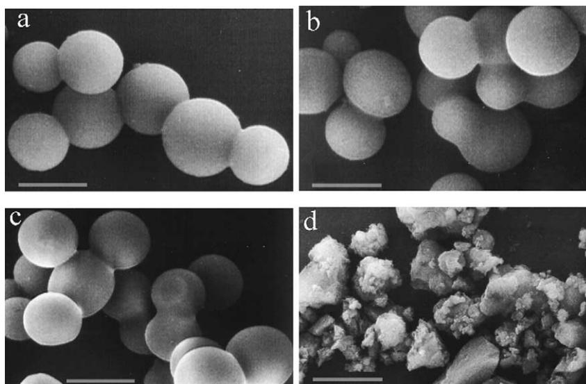
Fig. 1. SEM images of mesoporous  $\text{SiO}_2$  obtained at: (a) 80  $^{\circ}\text{C}$  for 5 h ( $\text{SiO}_2$ -1); (b) 80  $^{\circ}\text{C}$  for 5 h and 120  $^{\circ}\text{C}$  for 12 h ( $\text{SiO}_2$ -2); (c) 80  $^{\circ}\text{C}$  for 5 h and 130  $^{\circ}\text{C}$  for 12 h ( $\text{SiO}_2$ -3); (d) 130  $^{\circ}\text{C}$  for 12 h ( $\text{SiO}_2$ -4). Scale bar: 5  $\mu\text{m}$ .
