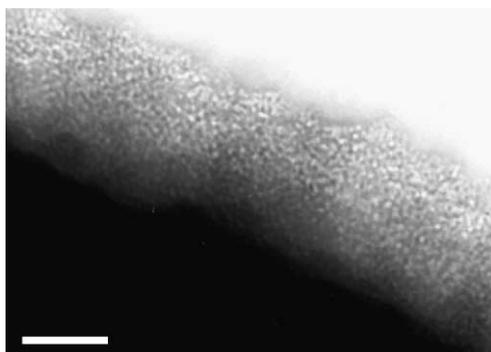
Fig. 5. TEM image of mesoporous silica spheres SiO<sub>2</sub>-2. Scale bar: 100 nm.
