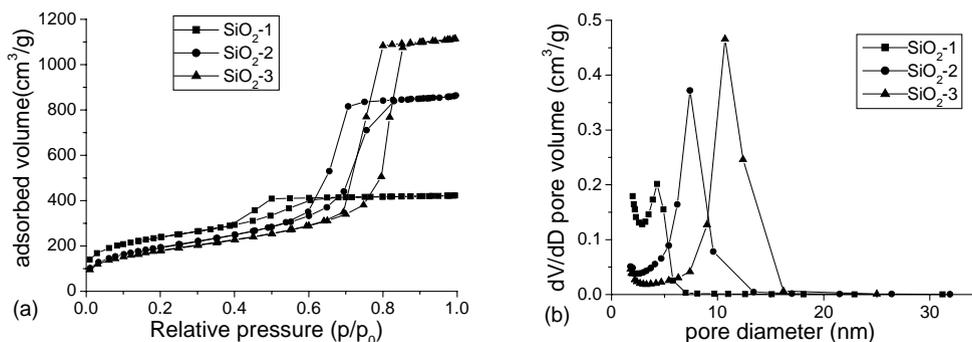
Fig. 4. N<sub>2</sub> adsorption–desorption isotherms (a) and pore size distribution curves from the adsorption branch (b) of mesoporous silica spheres.
