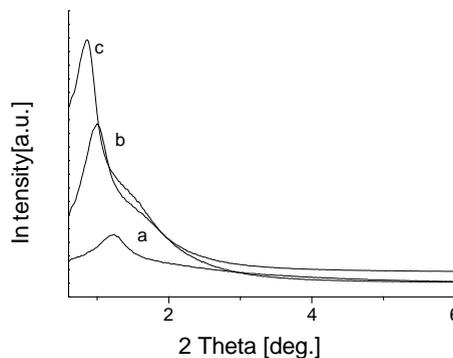
Fig. 3. XRD patterns of mesoporous silica spheres: (a) SiO<sub>2</sub>-1; (b) SiO<sub>2</sub>-2; (c) SiO<sub>2</sub>-3.
