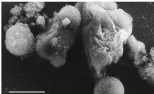
Fig. 2. SEM image of mesoporous SiO<sub>2</sub> synthesized in the absence of ethanol and under otherwise the same conditions as that of SiO<sub>2</sub>-3. Scale bar: 5 μm.
