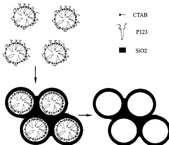
Fig. 6. Schematic diagram showing the assembly of the mixed P123–CTAB micelles and the formation of the final mesopore structure.
