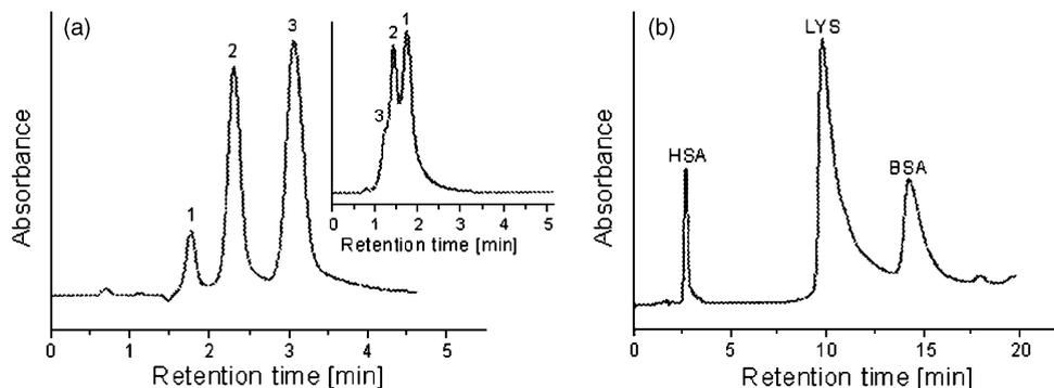
Fig. 10. Chromatograms of three aromatic molecules (a) and three proteins (b) with a  $SiO_2$ -2- $C_{18}$  column. Inset in (a) shows chromatogram of aromatic molecules with a  $SiO_2$ -2 column. Peaks 1–3 in (a) correspond to naphthalene, biphenyl, and phenanthrene, respectively, whereas the three peaks in (b) correspond to human serum albumin (HSA), lysozyme (LYS), and bovine serum albumin (BSA), respectively.
