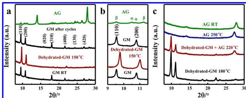
**Figure 3.** In-situ VT-PXRD characterization of guanine monohydrate dehydration process. Panels (a) and (b) reversible hydration/dehydration processes between dehydrated-GM (150 °C) and GM after a few dehydration hydration cycles, (c) irreversible process of dehydrated-GM to AG.
