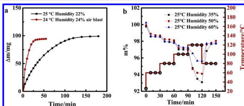
**Figure 6.** Characterizations on the hydration/dehydration process of GM in large scale. (a) About 1.5 g of GM treated at 120 °C was then exposed to air at RT, and the increasing weight of dehydrated-GM was recorded with time under standing and air blowing conditions. (b) The dehydration/hydration process of 1.5 g of GM was tested at different humidities and different temperatures, while the O locations were the measurement points for recording the sample weight.
