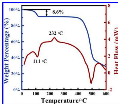
**Figure 2.** Characterizations of GM nanofibers by using DSC-TGA.
