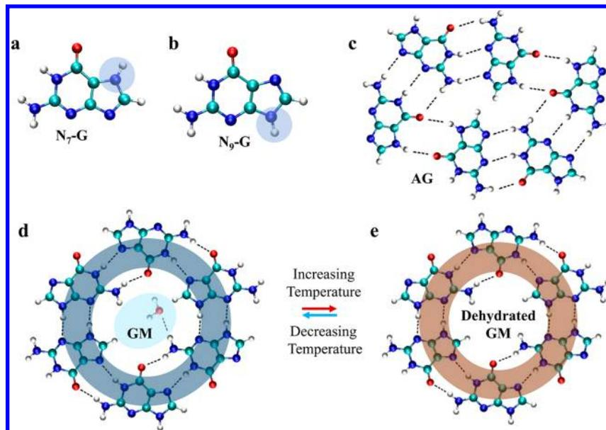
dehydrated-GM is monoclinic crystal composed of  $N_9$ -G, tautomeric polymorph of AG ( $N_7$ -G). The dehydrated-GM has long-term stability at room temperature and robust stability after repetitive water harvest from atmospheric air. Reversible and efficient dehydration/hydration transformation between GM and dehydrated-GM can proceed in large scale, probably due to their similar crystal structures and the elaborate water channels composed of six  $N_9$ -G molecules.
