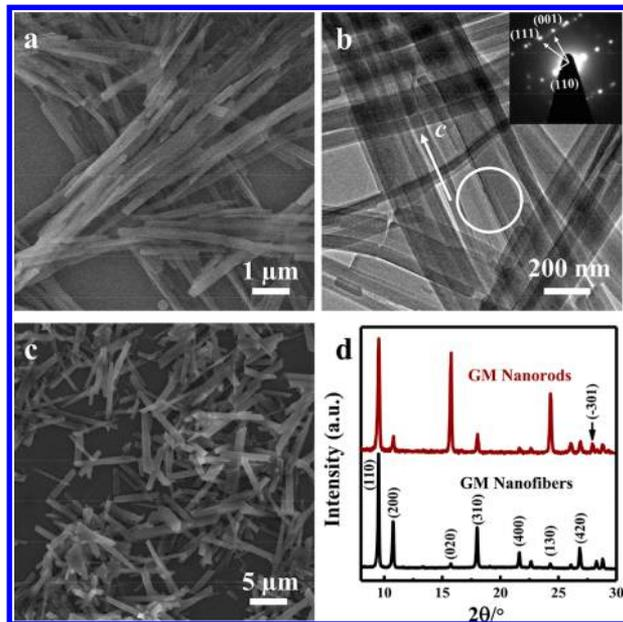
**Figure 1.** Characterizations of GM by using SEM, TEM, and PXRD. (a) SEM and (b) TEM images and SAED pattern (b inset) of single crystalline GM nanofibers obtained in acidic solution. (c) SEM image of GM nanorods obtained in PBS buffer with the presence of 2.7 mmol·L<sup>-1</sup> CTAB. (d) Powder X-ray diffraction (PXRD) of GM nanofibers and nanorods.
