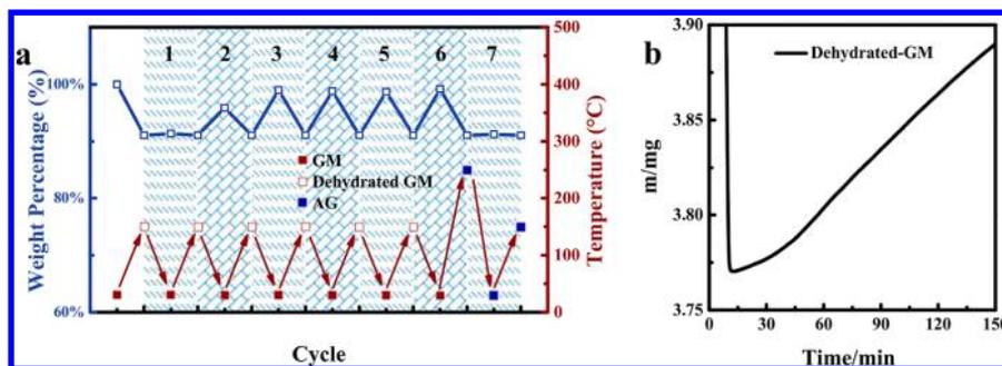
**Figure 5.** Characterizations on the hydration/dehydration process of GM in small scale. (a) Reversible water absorption ability of dehydrated-GM from atmospheric air. (b) Dehydrated-GM formed at 150 °C from GM was kept in a very dry furnace body (below 20% humidity), and the weight of the guanine was recorded with time.
