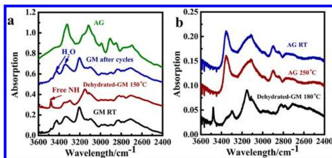
**Figure 4.** In-situ VT-FTIR spectroscopy of guanine monohydrate dehydration process. (a) Reversible hydration/dehydration processes between dehydrated-GM (150 °C) and GM after a few dehydration hydration cycles, (b) irreversible process of dehydrated-GM to AG.
