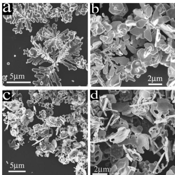
**Figure 5.** SEM images of Ag crystals formed in the presence of anionic DexS-40 at 60 °C.  $[\text{AgNO}_3] = 20 \text{ mM}$ .  $[\text{DexS-40}]$ : (a) 1, (b) 10, and (c,d) 100  $\text{g L}^{-1}$ .
