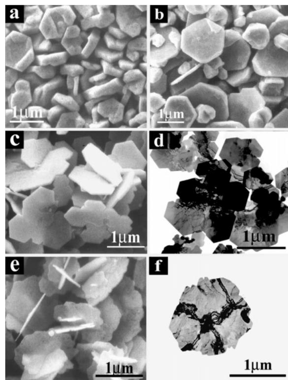
**Figure 6.** SEM (a–c,e) and TEM (d,f) images of Ag microdisks formed in mixed water–formamide solvents in the presence of anionic DexS-40 at 20 °C.  $[\text{AgNO}_3] = 2 \text{ mM}$ , and  $[\text{DexS-40}] = 10 \text{ g L}^{-1}$ . Formamide content (v %): (a) 0, (b) 10, (c,d) 50, and (e,f) 98.
