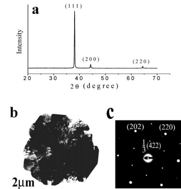
**Figure 4.** XRD pattern (a), TEM image (b), and ED pattern (c) of Ag microdisks formed in the presence of anionic DexS-40 at 20 °C.  $[\text{AgNO}_3] = 20 \text{ mM}$ , and  $[\text{DexS-40}] = 100 \text{ g L}^{-1}$ .
