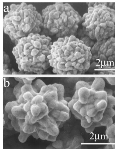
**Figure 2.** SEM images of Ag crystals formed at 20 (a) and 60 °C (b) in the presence of nonionic Dex-40.  $[\text{AgNO}_3] = 20 \text{ mM}$ , and  $[\text{Dex-40}] = 10 \text{ g L}^{-1}$ .
