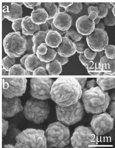
**Figure 1.** SEM images of Ag crystals formed at 20 (a) and 60 °C (b) in the absence of dextrans.  $[\text{AgNO}_3] = 20 \text{ mM}$ .
