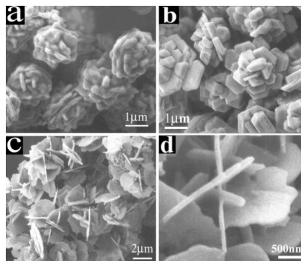
**Figure 3.** SEM images of Ag crystals formed in the presence of anionic DexS-40 at 20 °C.  $[\text{AgNO}_3] = 20 \text{ mM}$ .  $[\text{DexS-40}]$ : (a) 1, (b) 10, and (c,d) 100  $\text{g L}^{-1}$ .
