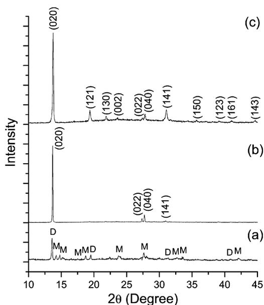
**Fig. 2** XRD patterns of strontium oxalate crystals obtained in the absence (a) and the presence (b,c) of PMAA. [PMAA]: (a) 0, (b) 0.126, (c) 1.26 g L<sup>-1</sup>. Peaks characteristic of SOM and SOD are labeled as 'M' and 'D', respectively. The indexed peaks are from SOD.
