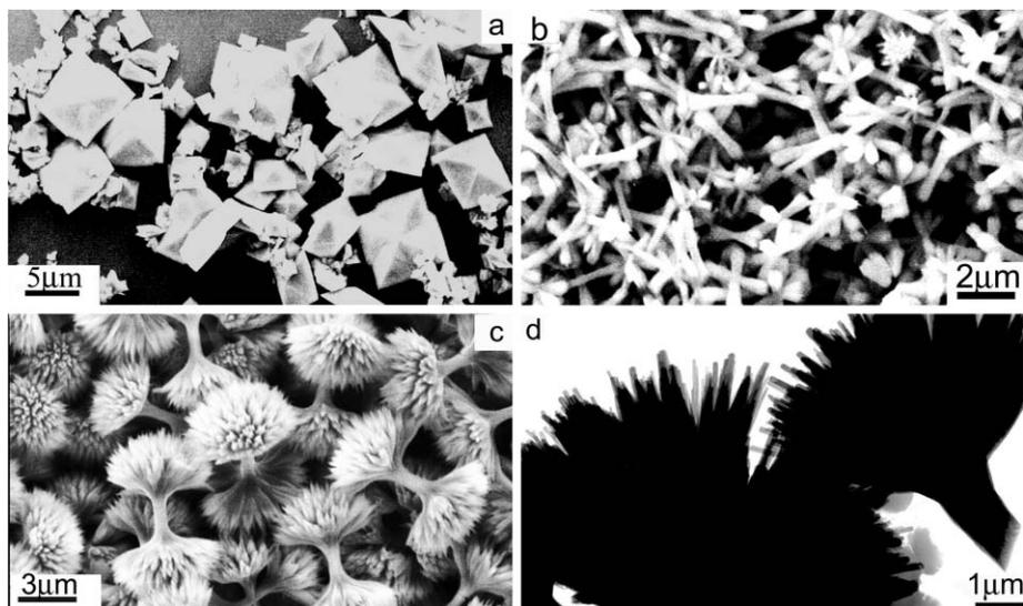
**Fig. 1** SEM (a–c) and TEM (d) images of strontium oxalate crystals obtained in the absence (a) and the presence (b–d) of PMAA. [PMAA]: (a) 0, (b) 0.126, (c,d) 1.26 g L<sup>-1</sup>.
