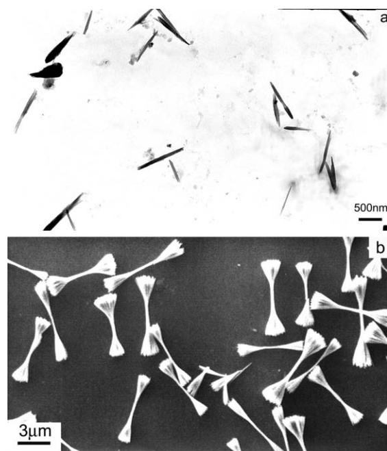
**Fig. 3** TEM (a) and SEM (b) micrographs of strontium oxalate crystals obtained in the presence of PMAA. Aging time: (a) 20 min, (b) 5 h; [PMAA] = 1.26 g L<sup>-1</sup>.
