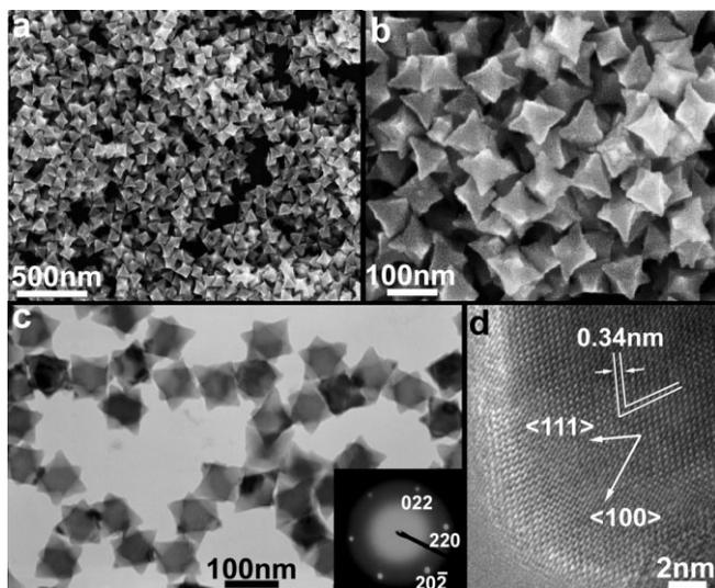
**Figure 1.** a,b) SEM, c) transmission electron microscopy (TEM), and d) high-resolution TEM images of star-shaped PbS nanocrystals obtained in mixed CTAB/SDS solution after a reaction time of 5 h. The inset in (c) shows the electron diffraction (ED) pattern obtained from an individual PbS star.
