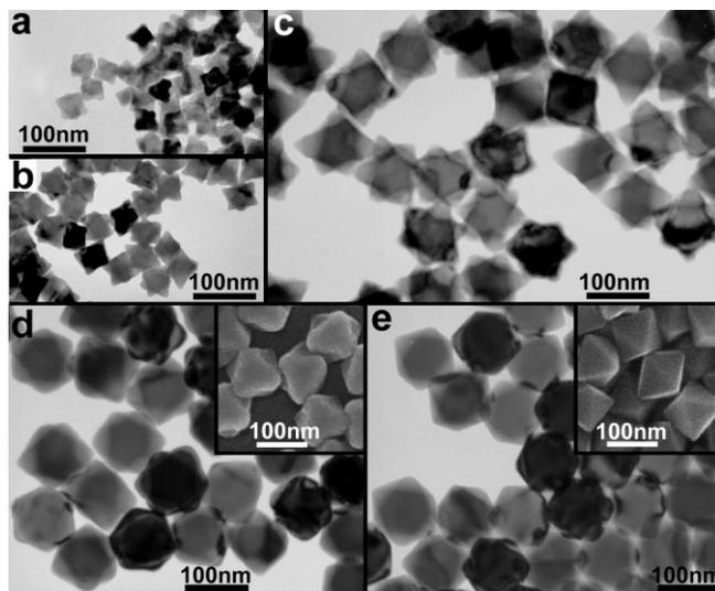
**Figure 2.** TEM images of PbS nanocrystals obtained in mixed CTAB/SDS solution after reaction times of: a) 1 h, b) 2 h, c) 12 h, d) 1 day, and e) 2 days. Insets in (d,e) show the corresponding SEM images.
