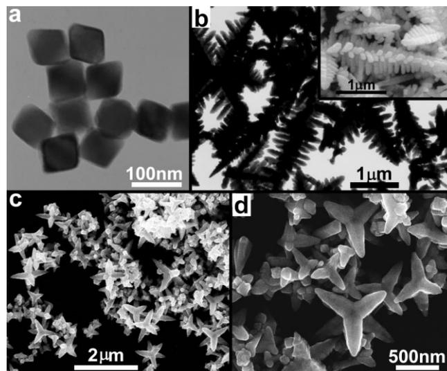
**Figure 4.** a,b) TEM and c,d) SEM images of PbS crystals obtained in single CTAB (a) and SDS solution (b–d): a) [CTAB]=5.7 mM, 5 h; b) [SDS]=1.1 mM, 5 h; c,d) [SDS]=11 mM, 14 h. The inset in (b) shows the corresponding SEM image.
