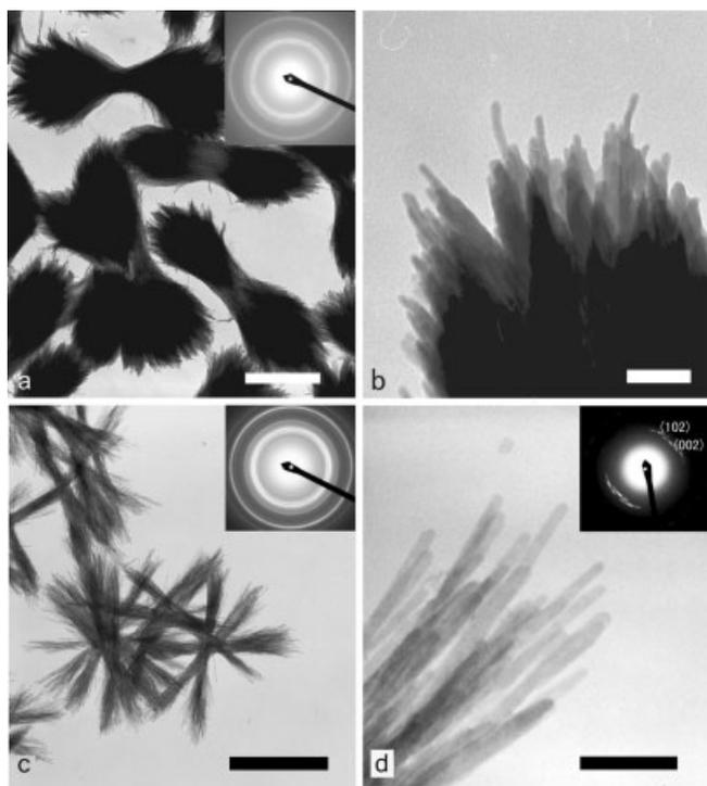
Fig. 1. TEM images of BaCrO<sub>4</sub> nanowires formed at 30 °C and  $r = 1$  (a,b) and  $r = 0.4$  (c,d). Insets show the corresponding ED patterns. Scale bars: a) 500 nm, b) 50 nm, c) 1 μm, d) 100 nm.
