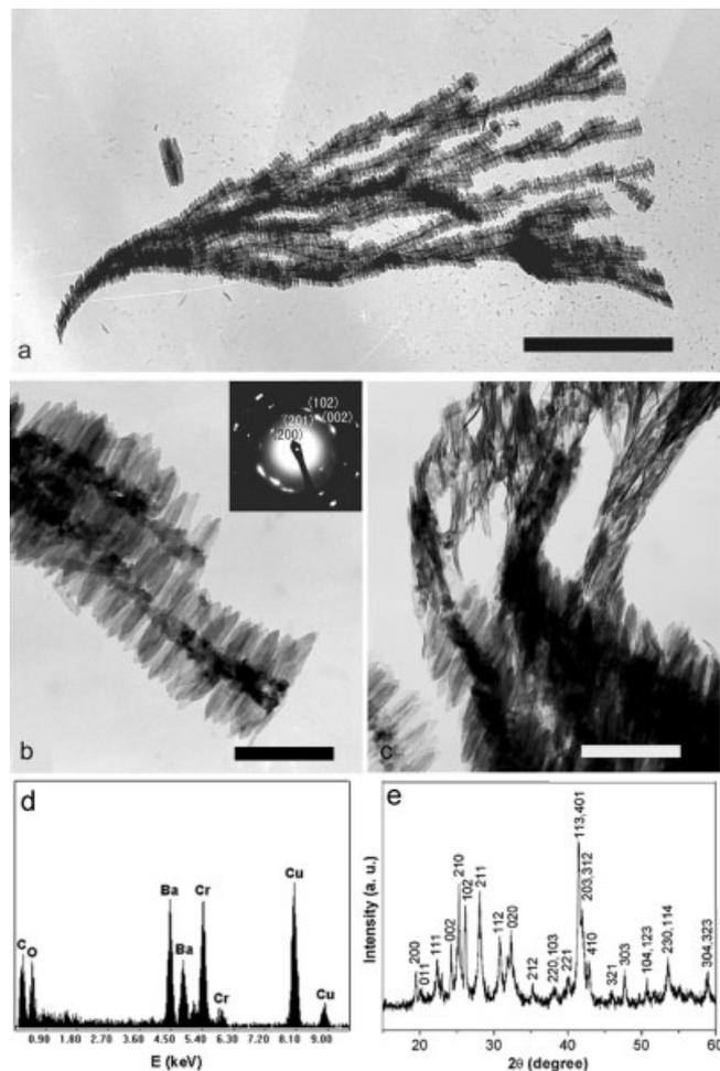
Fig. 3. TEM images (a–c), EDS spectrum (d), and XRD pattern (e) of tree-like BaCrO<sub>4</sub> superstructures formed at 30 °C and *r* = 1.7. Inset shows the corresponding ED pattern. Scale bars: a) 2 μm, b,c) 200 nm.
