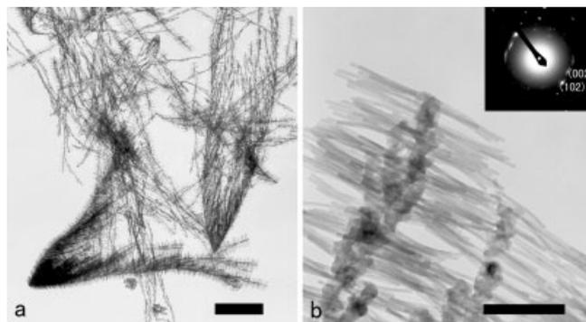
Fig. 6. TEM images of BaCrO<sub>4</sub> nanostructures formed at 50 °C and  $r=1.7$ . Insets show the corresponding ED patterns. Scale bars: a) 2 μm, b) 200 nm.
