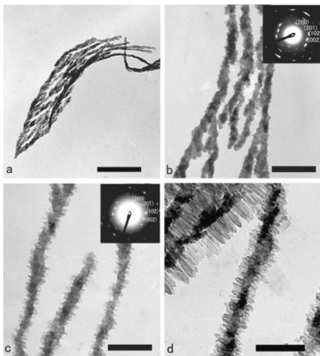
Fig. 5. TEM images of BaCrO<sub>4</sub> nanostructures obtained at earlier stages for the tree-like superstructures formed at 30 °C and  $r=1.7$ . Aging time: a,b) 5 min, c) 15 min, d) 8 h. Insets show the corresponding ED patterns. Scale bars: a) 500 nm, b–d) 200 nm.
