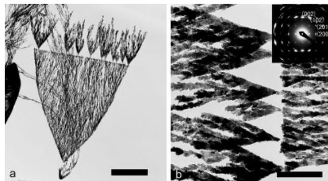
Fig. 4. TEM images of bare-tree-like BaCrO<sub>4</sub> superstructures formed at *r* = 2. Inset shows the corresponding ED pattern. Scale bars: a) 2 μm, b) 500 nm.
