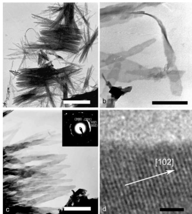
Fig. 2. TEM images of BaCrO<sub>4</sub> nanobelts formed at 30 °C and  $r = 1.4$ . Inset shows the corresponding ED pattern. Scale bars: a) 1 μm, b,c) 200 nm, d) 2 nm.
