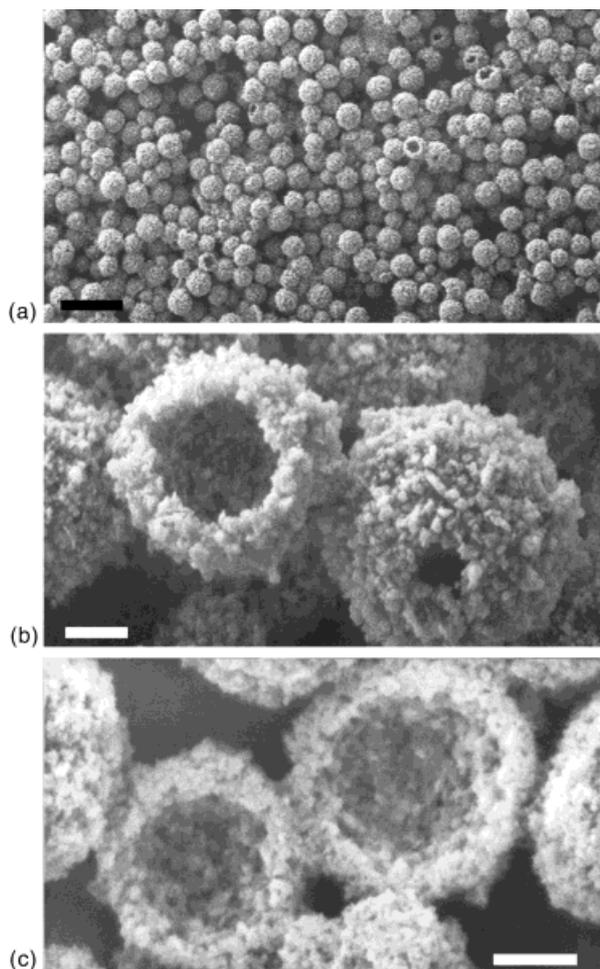
Fig. 1. a) SEM image of calcite hollow spheres formed in mixed PEO-*b*-PMAA-SDS solutions before sonication. b) High-magnification SEM image of two broken calcite hollow spheres. c) High-magnification SEM image of calcite hollow spheres after sonication. [SDS] = 2 mM. Scale bars: a) 10  $\mu\text{m}$ , b) 1  $\mu\text{m}$ , c) 1  $\mu\text{m}$ .
