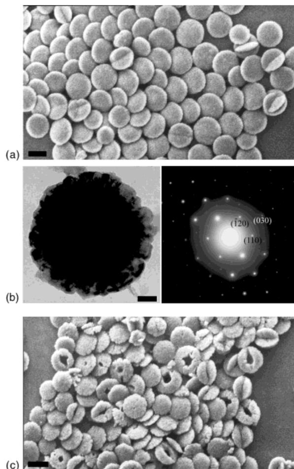
Fig. 2. SEM images of the vaterite discs formed in mixed PEO-*b*-PMAA-SDS solutions after 1 day (a,b) and 7 days (c) of aging. The ED pattern of the disc shown in (b) is presented on the right side of (b), which corresponds to the [001] zone of vaterite. [SDS] = 10 mM. Scale bars: a) 1  $\mu\text{m}$ , b) 0.2  $\mu\text{m}$ , c) 1  $\mu\text{m}$ .
