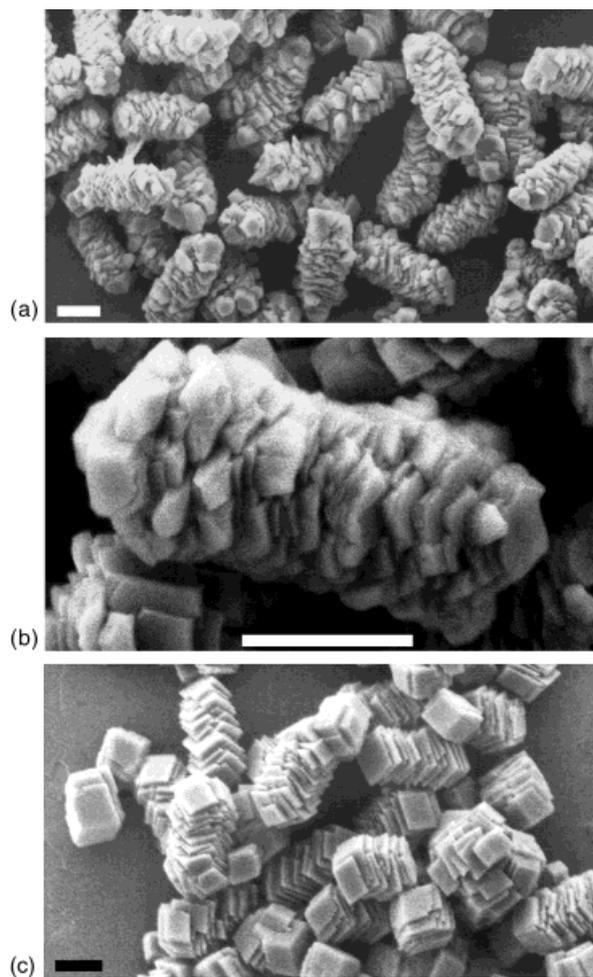
Fig. 3. SEM images of the calcite crystals formed in mixed PEO-*b*-PMAA-CTAB solutions. a,b) [CTAB] = 1 mM. c) [CTAB] = 2 mM. Scale bars =  $1 \mu\text{m}$ .
