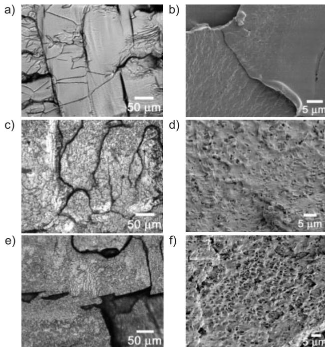
Fig. 4. a) Optical micrograph of PS impact specimen fracture surface. b) SEM of PS impact specimen fracture surface. c) Optical micrograph of PS/0.5 wt.-% DRC impact specimen fracture surface. d) SEM of PS/0.5 wt.-% DRC impact specimen fracture surface. e) Optical micrograph of PS/1.0 wt.-% DRC impact specimen fracture surface. f) SEM of PS/1.0 wt.-% DRC impact specimen fracture surface.
