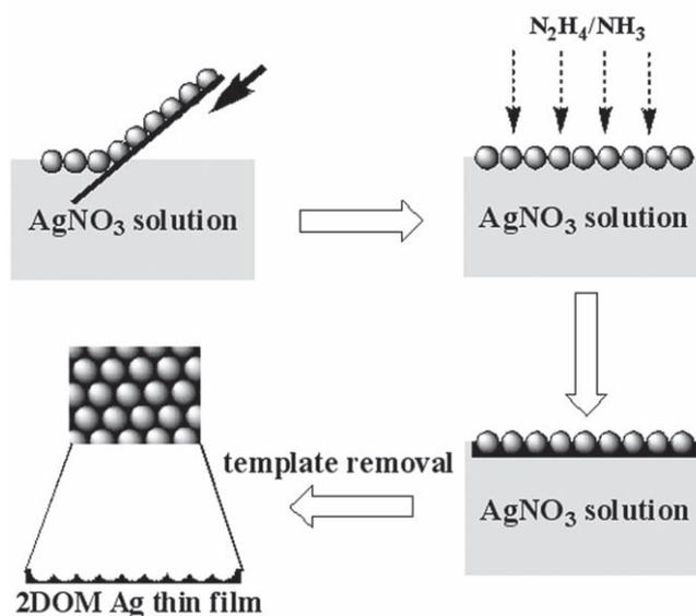
**Scheme 1.** Protocol for the preparation of 2DOM Ag thin film via the NSLSS method.
