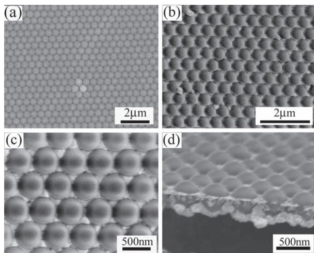
**Figure 2.** SEM images of 450 nm MCC template (a) and the templated MCC-Ag composite by top view (b,c) and side view (d).
