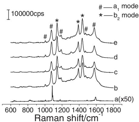
**Figure 3.** a) Raman spectrum of solid 4-ATP. b–e) SERS spectra of 4-ATP molecules adsorbed on the obverse side of 2DOM Ag thin films with different periodic spacings: b) 130 nm; c) 450 nm; d) 600 nm; e) 1000 nm.
