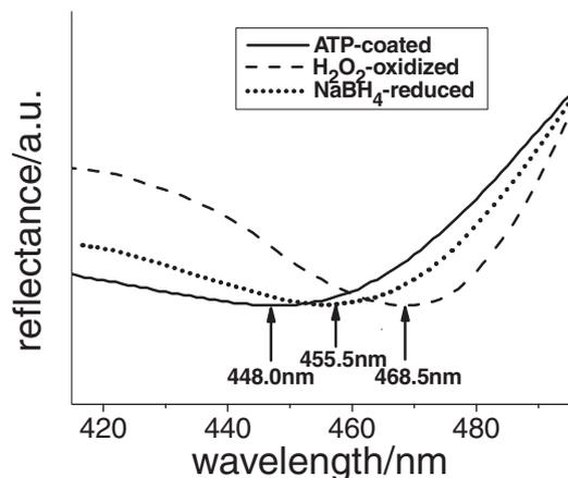
**Figure 4.** Reflectance spectra of 2DOM Ag thin films activated by modification with 4-ATP, oxidized by  $\text{H}_2\text{O}_2$ , and reduced by  $\text{NaBH}_4$ .
