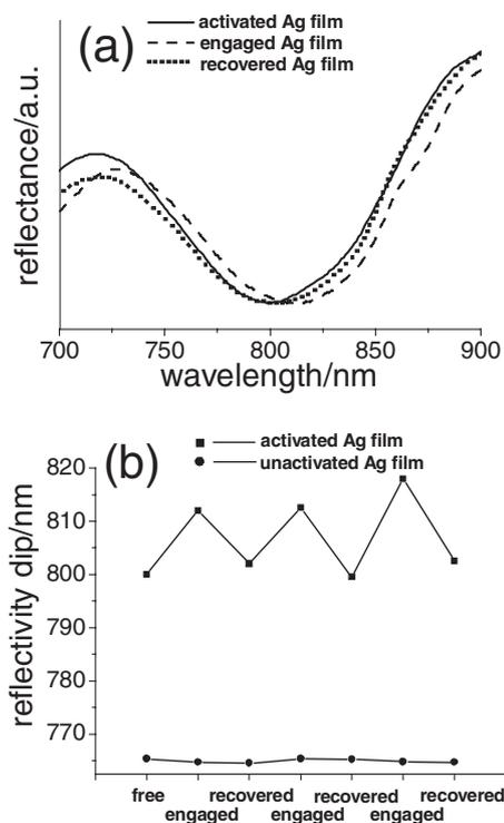
**Figure 5.** a) Reflectance spectra of 2DOM Ag thin films activated by modification with 3-MPA, engaged by adsorption of decylamine, and recovered by washing with acetic acid. b) Relationship between the reflectivity dip position and the status of the activated Ag thin films together with the variation of dip position with the status of the unactivated Ag thin films that were not treated with 3-MPA.
