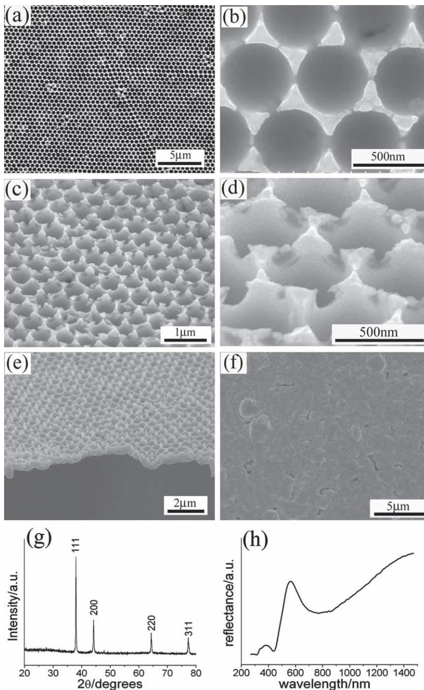
**Figure 1.** SEM images (a–f), XRD pattern (g), and reflection spectrum (h) of 2DOM Ag thin films with a periodic spacing of 450 nm. SEM images were observed from different directions: a,b) vertical top view; c,d) tilted top view; e) side view; f) bottom view.
