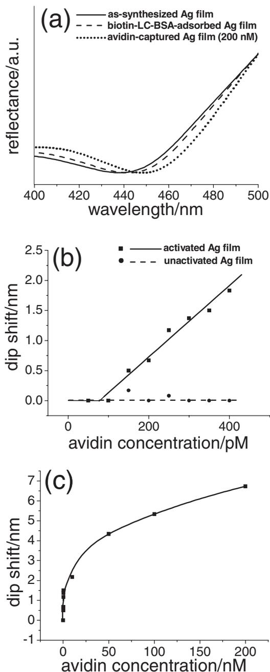
**Figure 6.** a) Reflectance spectra of 2DOM Ag thin film biosensors with different adsorbed molecules. b,c) Relationship between the reflectivity dip position and the avidin concentration in the concentration range of 0–400 pM (b) and the range of 0–200 nM (c). For comparison purpose, the situation of the unactivated Ag film without activation with biotin-LC-BSA is also shown in (b).
