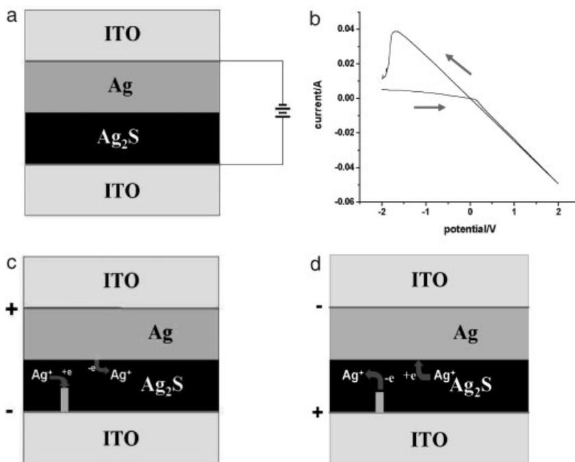
**Figure 8.** a) Schematic structure of the ITO/Ag/Ag<sub>2</sub>S/ITO device, and b) its *I*–*V* curve. c, d) Schematic drawings of the operating mechanism.
